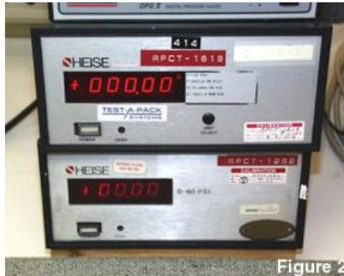
Note: If you are calibrating over the full range in In.H<sub>2</sub>O, you will need a calibration standard capable of measuring and displaying 1385.99 In.H<sub>2</sub>O.
